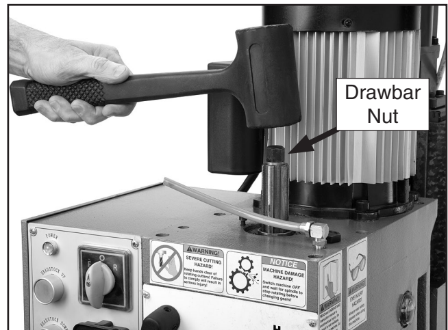
Figure 14. Unseating the arbor/cutter.
